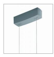
Wire suspension set with fast fine adjustment with clutch device (ZPH401/402 US) or screw device (ZPH301 US). Rectangular ceiling cap included. Available in white (WH) and silver (SI). Cable length 1500 mm, 1.2 mm<sup>2</sup>
